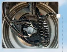
TRAILING-LINK CHASSIS SUSPENSION. Handles a full range of field loads and travel
