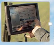
PORTABLE PRECISION CONTROL. AFS Pro 700 color display has a big bright screen and is faster, lighter and transferable to other Case IH machines. It allows the operator to easily control application rates and guidance functions.
