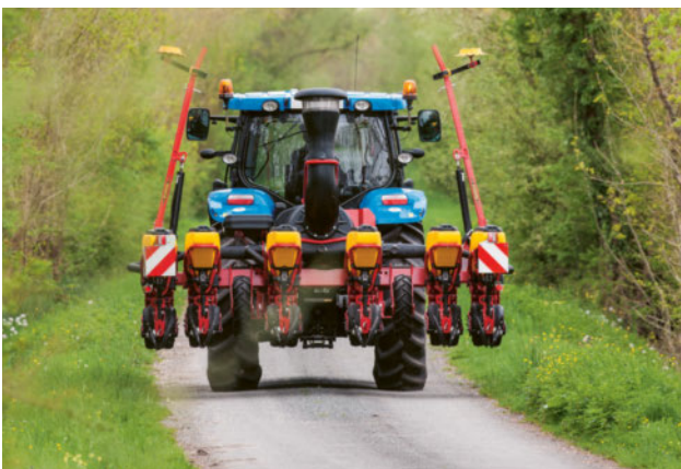
Tempo T has a transport width between 3.3 and 3.5 metres. This gives a small turning radius and convenient transport.
