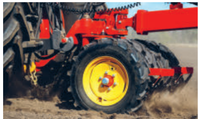
The pivot packer option consolidates the soil between the tractor wheels enabling each seed to have the same conditions for germination.
