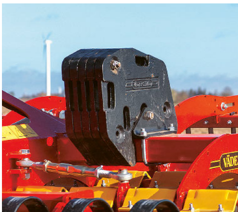
Carrier 300-400 can be equipped with weight packages resulting in up to 800kg/m.
