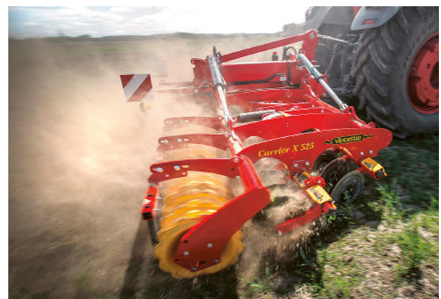
The working depth is set from the tractor cab, enabling adaptation to varying conditions in the field.
