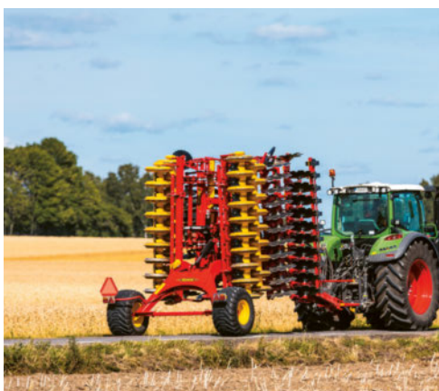
When transporting Carrier XL 425-625 between fields, the machine is wing-folded to fit within 3m transport width.
