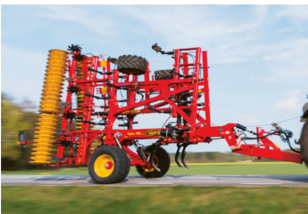
The carrying wheels positioned in the middle of the machine, makes Opus both easy to transport and gives it a small turning radius on headlands.
