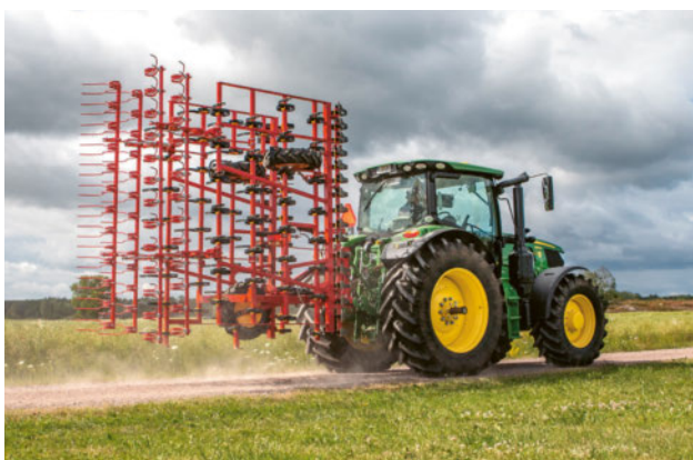
NZ Mounted folds to 2.05 metre transport width, ensuring convenient transport between fields.
