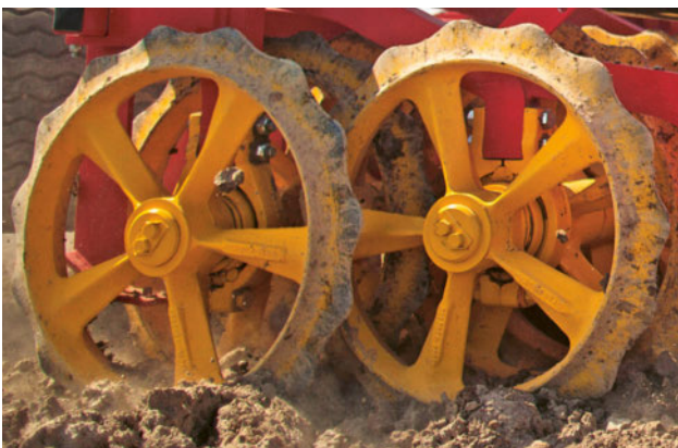
The packer rings are mounted in an offset position, minimising bulldozing and lowering the draught requirement.
