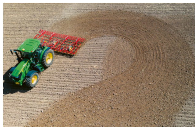
The unique versatile drawbar makes it possible to turn, with NZ Mounted in working position.
