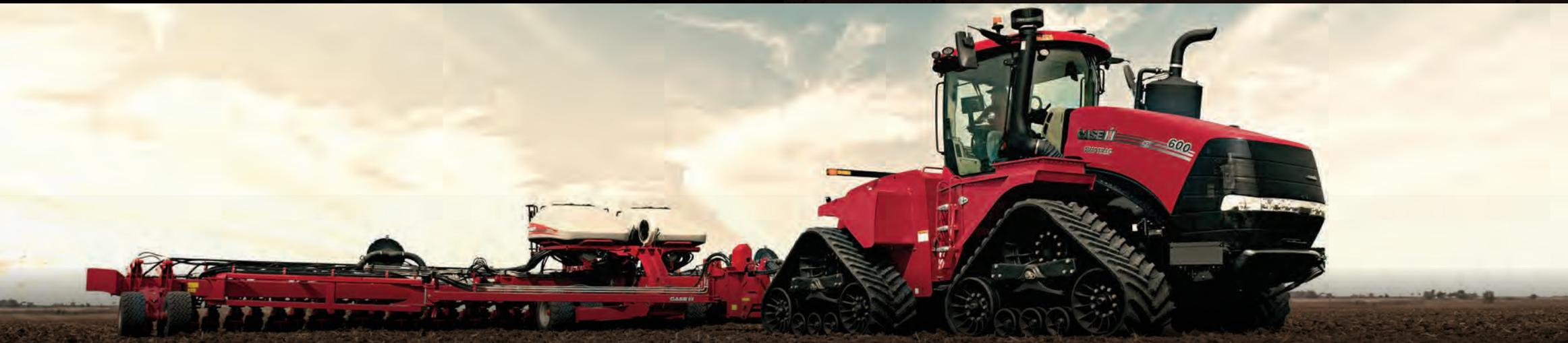
**QUADTRAC** | More than 20 years of industry-leading track technology can be found in every Steiger Quadtrac® AFS Connect tractor, which features four individually driven, positive-drive oscillating tracks.
